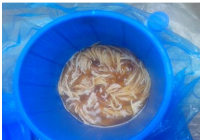
Figure 2: Soaking of Sisal fiber in NaOH
